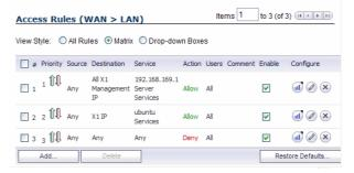
The access rules are sorted from the most specific at the top to the least specific at the bottom of the table. At the bottom of the table is the **Any** rule.
