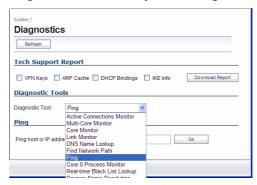
The Ping test bounces a packet off a machine on the Internet and returns it to the sender. This test shows if the SonicWALL security appliance is able to contact the remote host. If users on the LAN are having problems accessing services on the Internet, try pinging the DNS server, or another machine at the ISP location. If the test is unsuccessful, try pinging devices outside the ISP. If you can ping devices outside of the ISP, then the problem lies with the ISP connection.
