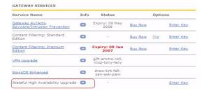
License synchronization is used during HA so that the Backup appliance can maintain the same level of network protection provided before the failover. To enable HA, you can use the SonicOS UI to configure your two appliances as a HA pair in Active/Idle mode.
