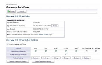
Select the Enable Inbound Inspection checkboxes for the protocols to inspect. By default, SonicWALL GAV inspects all inbound HTTP, FTP, IMAP, SMTP and POP3 traffic. CIFS/Netbios can optionally be enabled to allow shared access to files. Generic TCP Stream can optionally be enabled to inspect all other TCP based traffic, such as non-standard ports of operation for SMTP and POP3, and IM and P2P protocols.
