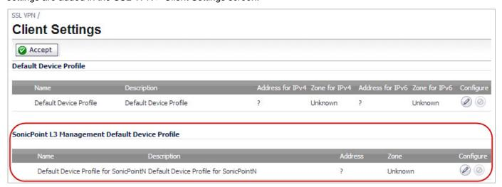
Just like the Device Profiles for other SonicOS firmware versions, this new Device Profile has the basic SSL VPN setting such as: Zone, Network Address, Client Setting, and Client Routes.
