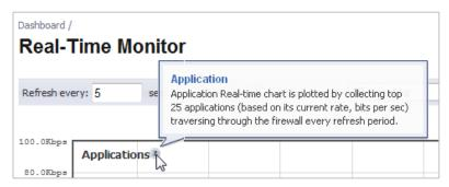
**Real-Time Monitor Collapse/Expand Options** — The **Dashboard > Real-Time Monitor** page provides a collapse/expand button for each chart. This allows the administrator to juxtapose two charts for comparison, even if they are normally far apart on the page.
