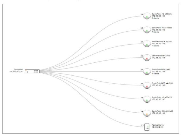
Topology View management provides a graphic presentation of the WLAN network for administrators with the most often used information and status. The devices are drawn as nodes on a tree and the tree is zoomable with the mouse and mouse wheel. Information shown in the tree includes device type, IP address, interface connected to, name, number of clients, and a simulated LED light on certain device shows working status. A tooltip bubble shows detailed information about a device.
