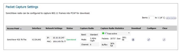
You can configure the mode, band and channel settings in the configuration dialog, allowing you to capture wireless packets in a specific channel. You can configure up to five source and destination MAC addresses.
