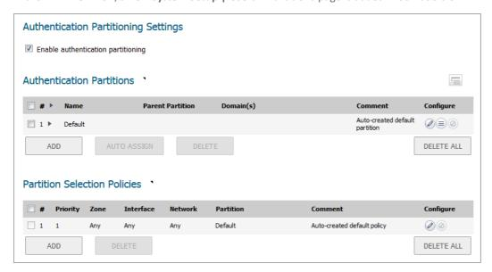
The partitions configured under **Authentication Partitions** control which authentication servers are used for which users, where those users are in different network partitions.
