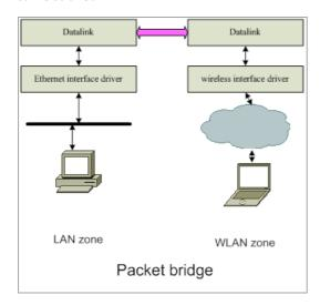
Previous versions of SonicOS provide L2 Bridge and Portshield support to provide some extent of Layer 2 bridging among LAN, WAN and other applicable zones. TZ Wireless and SOHO Wireless appliances support the WLAN Layer2 bridge feature. However, the WLAN Layer 2 bridge feature permits clients connected to the TZ/SOHO internal wireless to share an IP subnet with only LAN and DMZ zones, and only one-to-one Layer2 bridging is supported.
