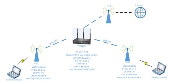
You can enable WDS mode for an access point by selecting the **Enable WDS AP** checkbox in the **Wireless > Base Settings** page or in the SonicWave/SonicPoint **Radio 0/1 Advanced** configuration. On the TZ or SOHO Wireless appliance, the **Enable Station Mode** and **Enable WDS Station** settings are available for configuring station mode.
