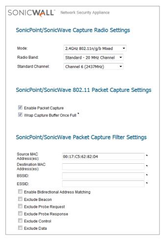
To capture the data for one of configured access point radios, click the **Download** button for that row on the **Access Points > Packet Capture** page. The capture file is named with the format, "wirelessCapture\_[SW name].cap", where "SW name" is the SonicWall access point name. Wireshark™ can be used to read the file.
