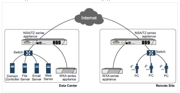
WAN acceleration using a SonicWALL WXA series appliance can provide an increase in application performance response time without purchasing a higher quality service or larger provision of bandwidth. This is especially noticeable on WAN connections such with high latency, which causes some applications to perform poorly.
