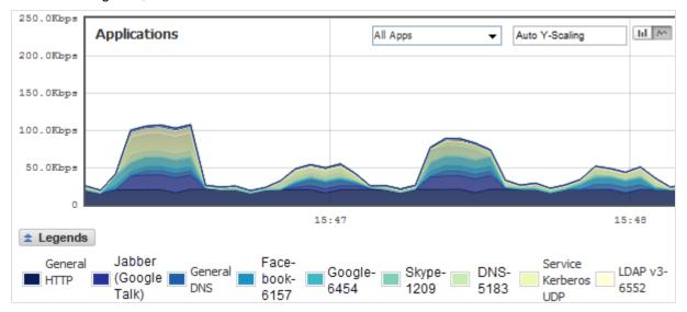
To relocate the legends into the Application or Bandwidth charts, click the icon, then select the desired checkbox(s).
