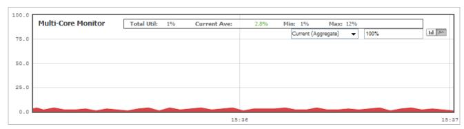
**Note**: In SonicOS 5.8.1.8, the Multi-Core Monitor only shows the processor load for the cores of the managing firewall. If operating in Active-Active DPI mode, the core load for the standby firewall does not display.
